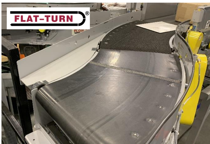
Two (2) S-curves in mirror-image design, each consisting of two (2) 45-degree Flat-Turn curves
