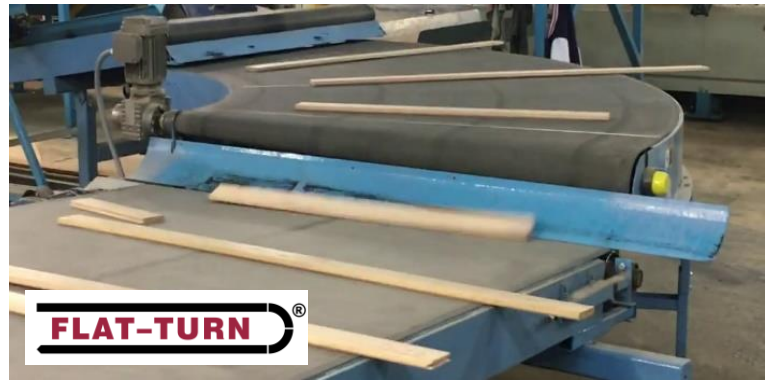
90-deg. Flat-Turn used in wood furniture production
