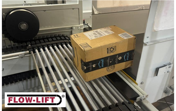
SKR Conveyor used as metering conveyor for a Flow-Lift S-Conveyor (CVC Continuous Vertical Conveyor)
