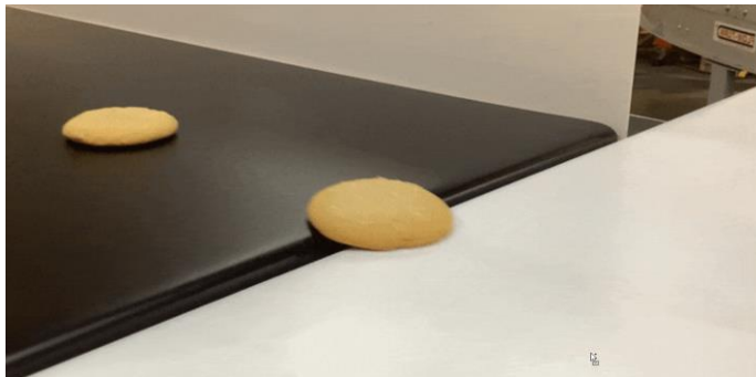
SKR Conveyor used as gapper conveyor, with integrated photo sensor and reflector. Gappers are typically installed in groups, e.g. six or nine gappers, to optimize sorter induction processes
