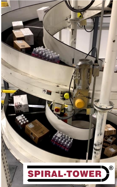
900-degree Spiral-Tower used in a liquor distribution center. Net elevation difference of 154", consisting of 2x 270-deg. and 2x 180-deg. spiral segments. (Model B-SP-SQ-24_35-900-154). Above right: Spiral-Turn segments prepared for truck shipment
