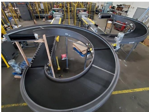
Two (2) 360-degree Spiral-Towers B-SP-SQ-34_25-360-52 in CCW-UP-3 configuration, consisting of two (2) Square-Turn Belt Spirals with 2.5" Dia. End Rolls, used in a bag packaging system
