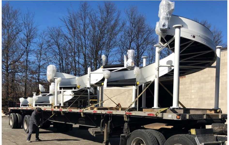
900-degree Spiral-Tower used in a liquor distribution center. Net elevation difference of 154", consisting of 2x 270-deg. and 2x 180-deg. spiral segments. (Model B-SP-SQ-24_35-900-154). Above right: Spiral-Turn segments prepared for truck shipment
