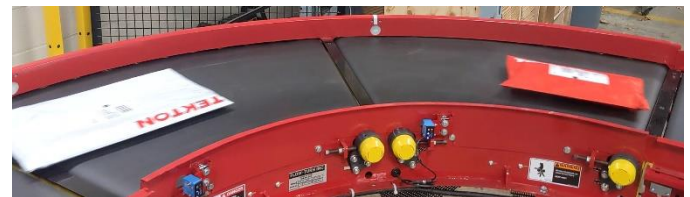
90-degree Double Zone-Turn Belted Curve with two 45-degree Zones (ZT2-32_27-90-P2)
